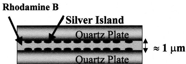
Fig. 2. Sample geometry. Two silver islanded quartz plates sandwich \approx 1 \mu\text{m} RhB solution. Given that metal-fluorophore interactions are thought to extend some 200 \text{ \AA} into the solution, in this sample geometry only \approx 4\% of RhB molecules are within this active region. This suggests that the true enhancement effect in Fig. 1 is at least 25 times higher.
